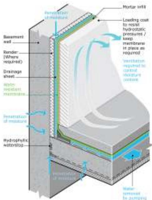
**Figure 6: Typical waterproofing requirements for a Grade 3/4 basement**
